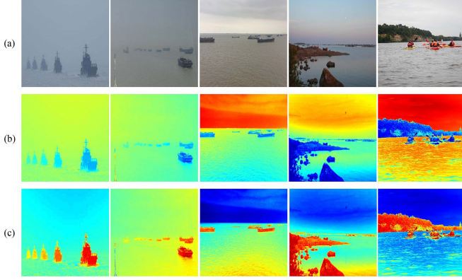
Fig. 3. Comparison of the (a) input image, (b) dark channel, and (c) inverted dark channel. To illustrate the distinctions more effectively, we utilize heatmaps for visualization.
